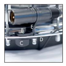
Put the screw into the connector hole and screw it. Place the connector on the resonator flange and let the screw pass through one flange hole. Fix the connector using the washer (D) and the nut (C).
