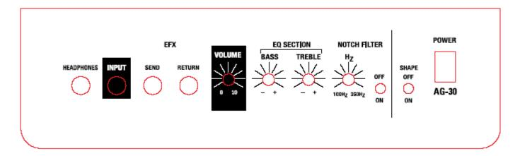
**HEADPHONES:** This jack provides a stereo signal to drive headphones. The use of this jack will disengage the amplifiers internal speaker.
