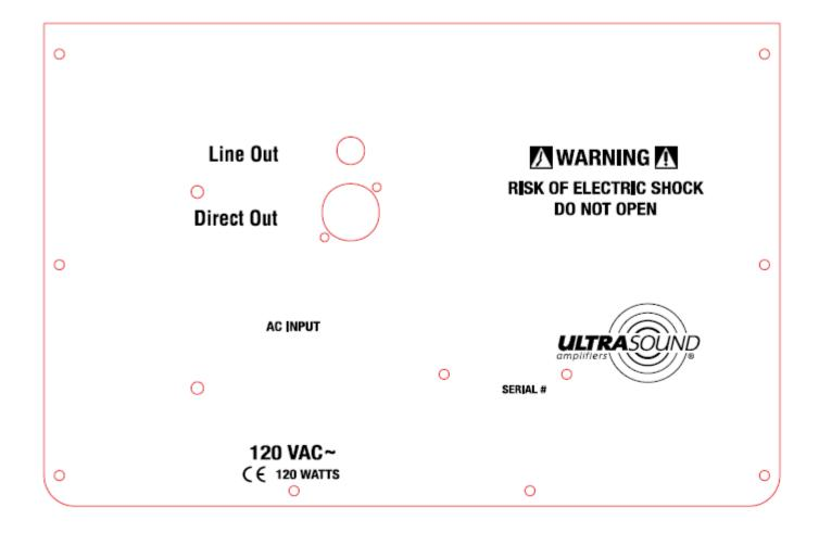
**AC INPUT:** Connect the female end of the AC line cord here. Connect the male plug to a suitable source of line voltage. Refer to the voltage information on the back of the amplifier for its voltage and current requirements. This connector also acts as the main fuse holder and includes a compartment for a spare fuse.
