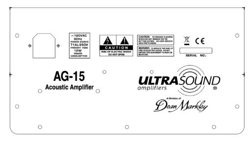
**AC INPUT:** Connect the female end of the AC line cord here. Connect the male plug to a suitable source of line voltage. Refer to the voltage information on the back of the amplifier for its voltage and current requirements. This connector also acts as the main fuse holder and includes a compartment for a spare fuse.
