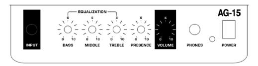
**INPUT:** Instrument input. Designed for both active and passive pickups.
