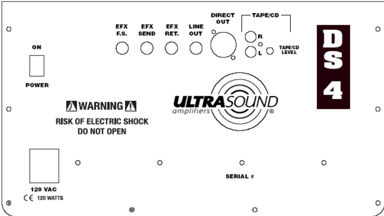
**EFX F.S. (FOOTSWITCH):** This jack is for connection to a shorting footswitch. When the switch is closed, the on board digital EFX will be bypassed.
